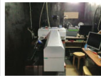
The **spectrometer** was realigned in summer 2012 with the help of TCCON community. The site is automated to provide remote control of the instrument. Measurements are performed during the days under clear sky conditions.
