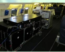
Lidar instrument in DC-8's cabin
