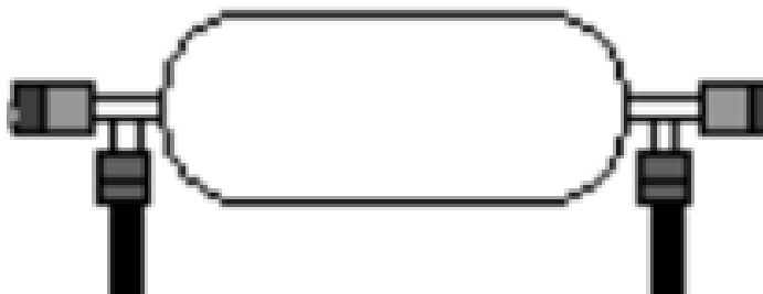
1.5L Pyrex glass vessel at \sim 0.12\text{MPa}
