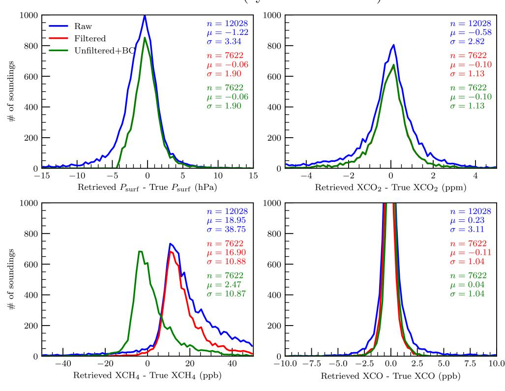
Random noise with a standard normal distribution may be applied using a proper noise model for a mapping grating spectrometer with noise coefficients for each band i:
