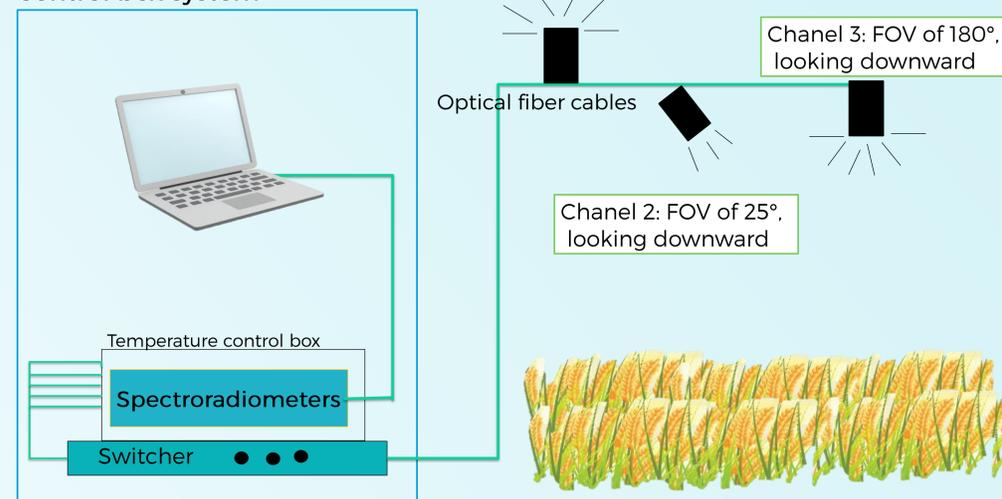
Figure 1. The Experimental system
