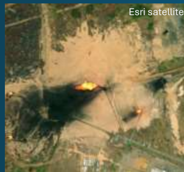
EnMAP detection at an O&G site, Punta de Mata, Venezuela. 9 Mar. 2025 Plume detection through the MARS Plume Viewer
