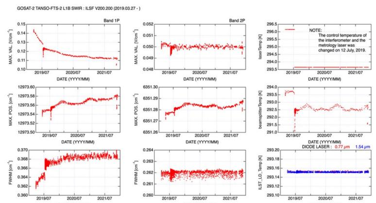
Fig. 5 Time series of the maximum value, its position, and FWHM of ILSF calibration.
