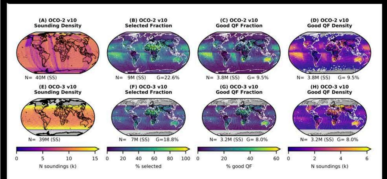
The polar orbit vs precessing orbit determine vastly different sampling patterns for OCO-2 (A) and OCO-3 (E). The L2FP prefiltering patterns, i.e., sounding selection, are similar (B and F), as are the patterns of good quality soundings (C) and (G), although differences exist due to filtering choices. The final density of good XCO2 retrievals are qualitatively similar for the overlapping latitude space (D and H).
