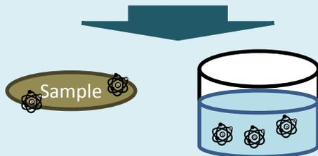
The sample and water are separated by filtration and the amount of radioactive Cs leached into the solution is determined.
