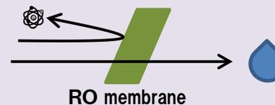
Radioactive Cs can be removed efficiently by using RO membrane filtration. However, residual water from the filtration contains highly-concentrated radioactive Cs. Proper management of this residual water is mandatory.
