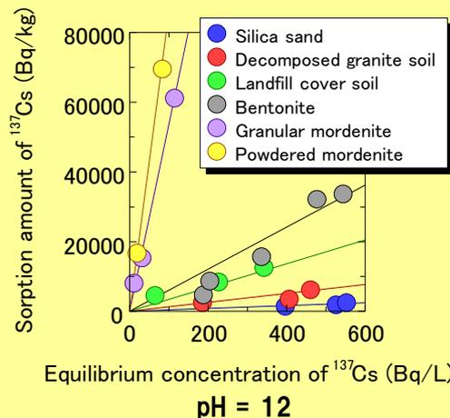
The two figures on the left show the results of a soil sorption test with Cs 137. The solution in the figure on the left is neutral (pH=7), the solution in the figure on the right is alkaline (pH=12). The horizontal axes of both figures are the mean equilibrium activities of Cs 137, and vertical axes are the mean adsorbed amount of Cs 137. **The steeper the slope of the relationship, the higher the sorptive capacity of the sample material.**
