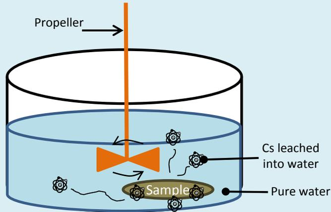
First, the sample is placed in a plastic container with an amount of pure water (equal to ten times the volume/weight of the sample). Then, the water is stirred for 6 hours.
