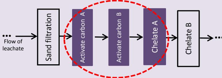
Mordenite was placed into these three filtration unit and leachate was treated for 24 hours
