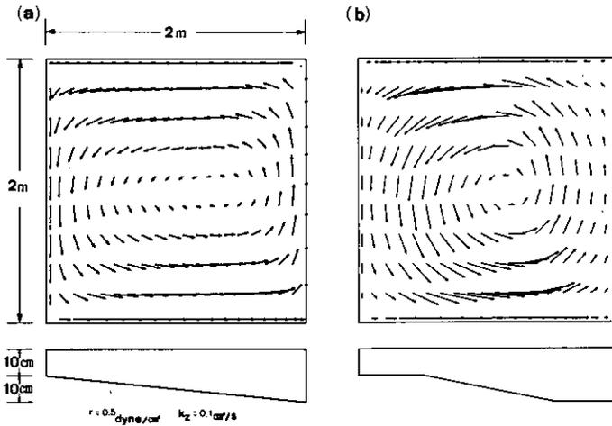
図 4-1 Ekman-type model 数値計算結果 ( $\tau_{wind} = 0.5 \text{ dyne/cm}^2$ ,  $K_z = 0.1 \text{ cm}^2/\text{s}$ )
