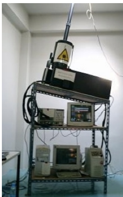
Polarization-sensitive (wavelength 532 nm) Mie-scattering (532 and 1064 nm) and Raman-scattering (607 nm) lidar system installed in Phimai, Thailand
