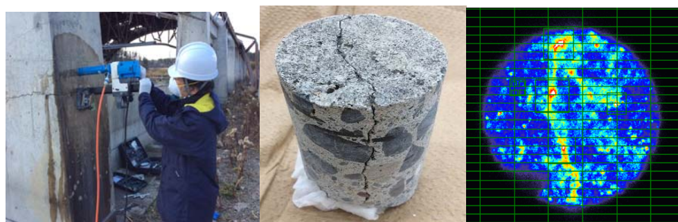
Fig. 4 Radioactive cesium contamination of concrete (diameter of plug: 5 cm)
