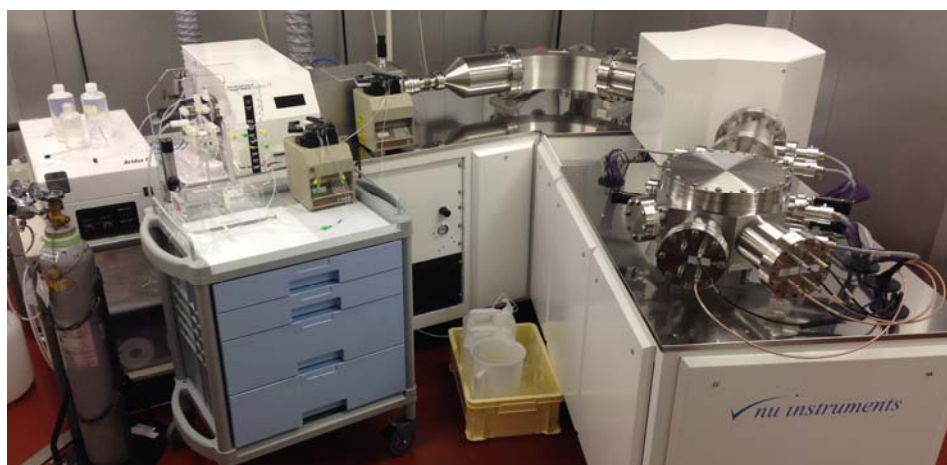
Cold-vapor generator coupled to a multi-collector inductively coupled plasma mass spectrometer, used to measure Hg isotopic ratios
