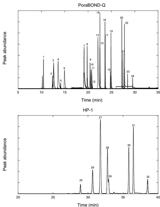
High-resolution analysis of halocarbons by multidimensional gas chromatography. Top: PoraBOND-Q column; bottom: thick-film HP-1 column.
