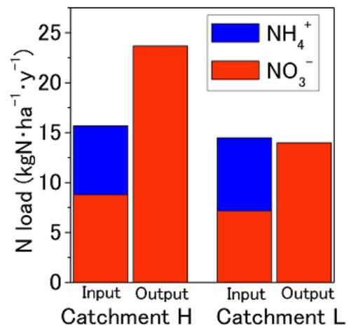
Clockwise from top left: view of Mt. Tsukuba; rainwater sampler in one of the test catchments at Mt. Tsukuba; comparison of the observed annual inorganic nitrogen budgets in the two test catchments, which have different nitrate-nitrogen concentrations in their baseflows formed by groundwater discharging to streams (annual average concentration of nitrate-nitrogen: 1.3 ppm N in catchment H and 0.50 ppm N in catchment L); and sampling of stream water.
