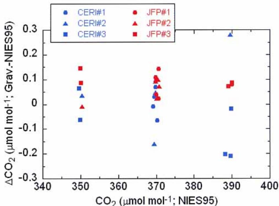
of the differences between the gravimetric and NDIR values (gravimetric – NDIR) were  $-0.00 \pm 0.13 \mu\text{mol mol}^{-1}$  for CERI and  $0.08 \pm 0.04 \mu\text{mol mol}^{-1}$  for JFP. These results suggest that the one-step dilution method is capable of preparing  $\text{CO}_2$  standards within an uncertainty of about  $\pm 0.1 \mu\text{mol mol}^{-1}$ .
