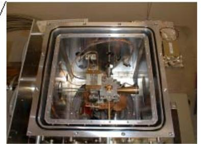
Millimeter Wave Ozone Spectrometer
