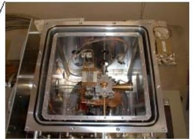
Millimeter Wave Ozone Spectrometer
