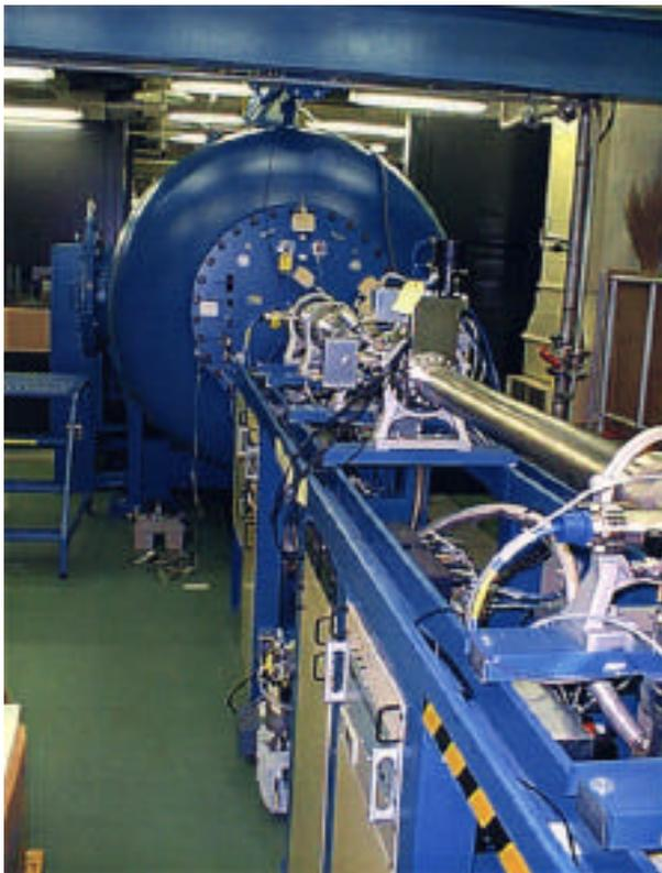
High voltage generator of accelerator mass spectrometer
