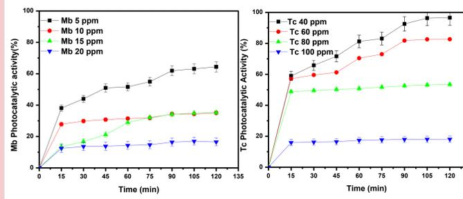
Figure 8. The rate of photo-catalytic activity of UV/ TiO<sub>2</sub> on concentrations of methylene blue and tetracycline. Total reaction time = 120 min; temperature= 25°C; Volume of the sample solution= 200mL; absorbance wavelength for methylene blue =664 nm, tetracycline= 357 nm, UV Lamp=360W; exposure time intervals = 15 min
