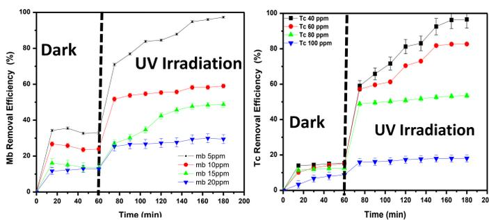
Figure 9. The effect of initial concentration on Mb and TC removal efficiency. Mb concentration= 5,10,15,20 ppm; Tc concentration= 40,60,80,100 ppm; Mb absorbance = 664 nm; TC absorbance= 357nm; temperature= 25°C, total reaction time=3 hr
