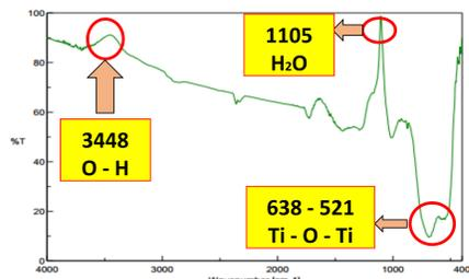
Figure 6. The Fourier transform infrared spectra of TiO<sub>2</sub> material
