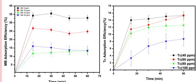
Figure 7. The TiO<sub>2</sub> adsorption efficiency test for different concentration of methylene blue and tetracycline. Total reaction time= 60 min; temperature= 25°C; Volume of the sample solution= 200mL; absorbance wavelength for methylene blue =664 nm, tetracycline= 357 nm
