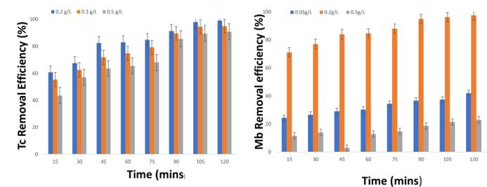
Figure 10. Effect of Catalyst dosage on the photocatalytic degradation of the optimized concentration of organic pollutants; Concentration of methylene blue= 5 ppm, Tetracycline= 40 ppm; catalyst=TiO<sub>2</sub> (0.2g/L, 0.3g/L, 0.5g/L); temperature= 25°C
