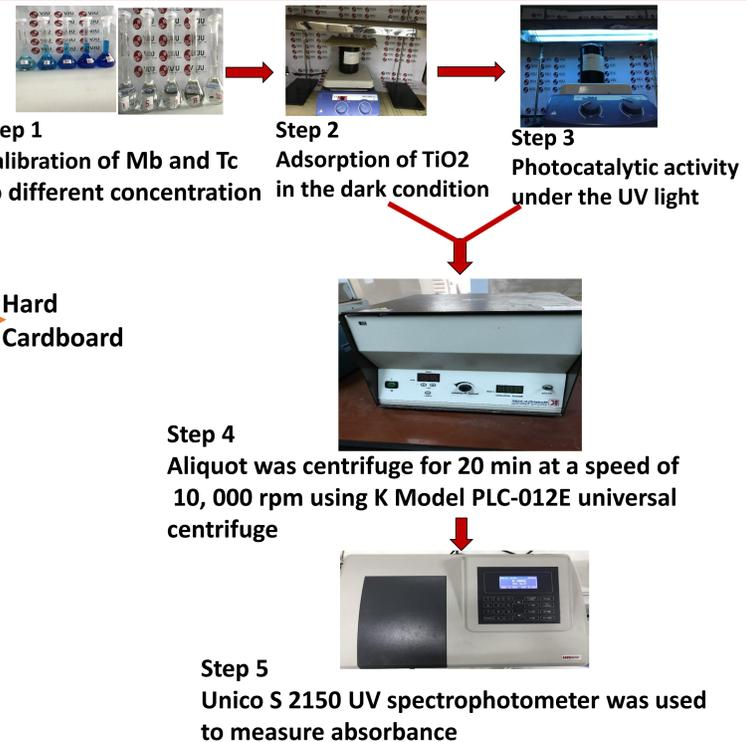
Figure 3. The overall process of the photocatalytic experiment
