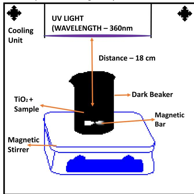
Figure 2. Schematic illustration of the set-up of the photocatalytic experiment
