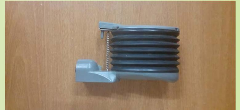
Old and New pumps for Dragger Detector tubes
