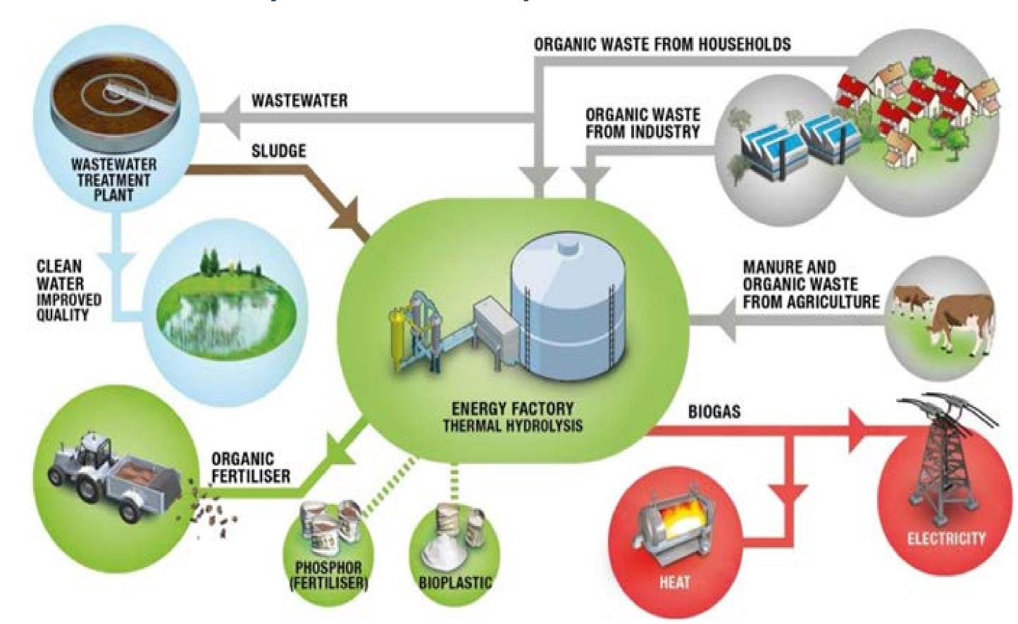
The "Recycling City" model, in which the city is integrated with "Zero waste agriculture" - Billund Bio Refinery Plant
