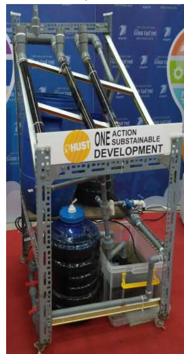
Figure 1. Solution for textile wastewater treatment by the porous PVA/AC-Fe(BDC) composite utilizing sunlight
