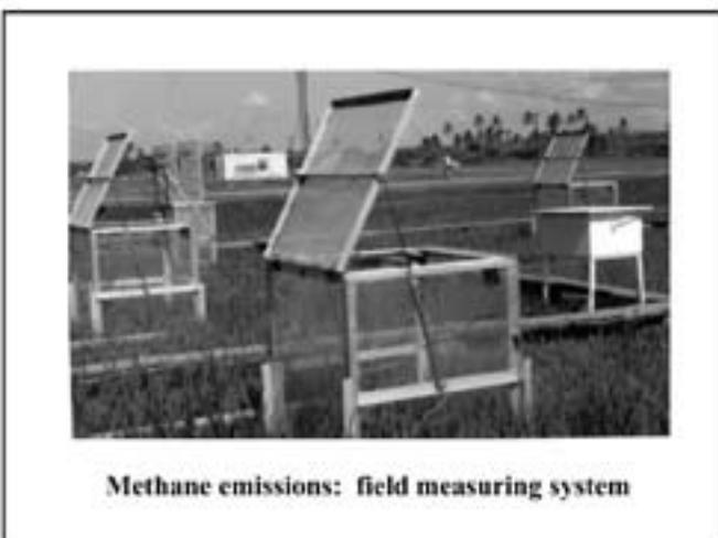
Methane emissions: field measuring system
