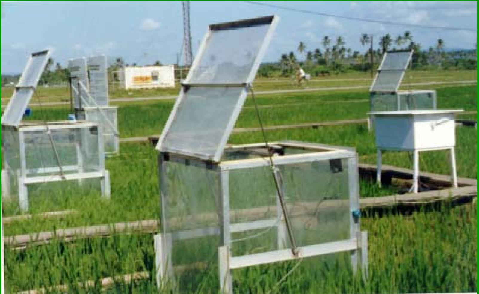
**Methane emissions: field measuring system**
