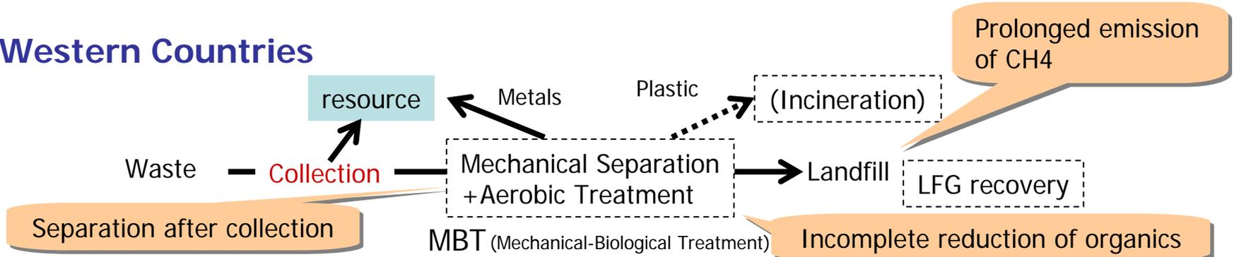
"Mechanical Separation" should be applicable to waste with low water content.
