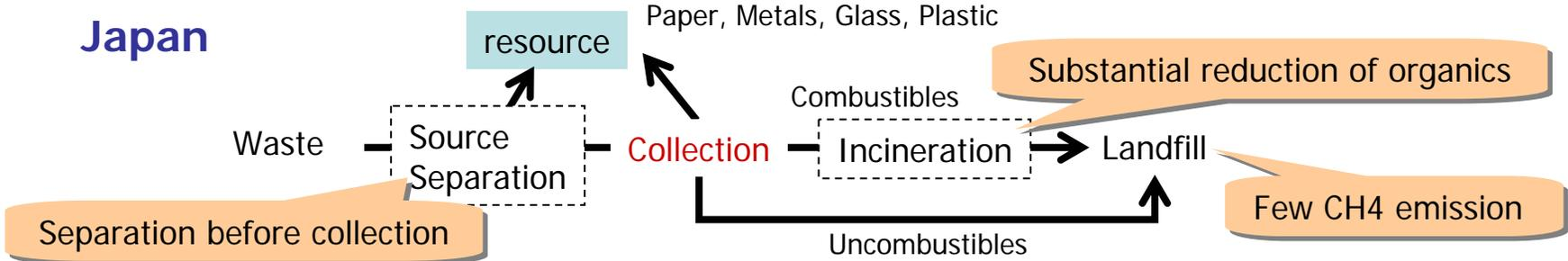
"Incineration" has been selected due to sanitation of waste with high water content.
