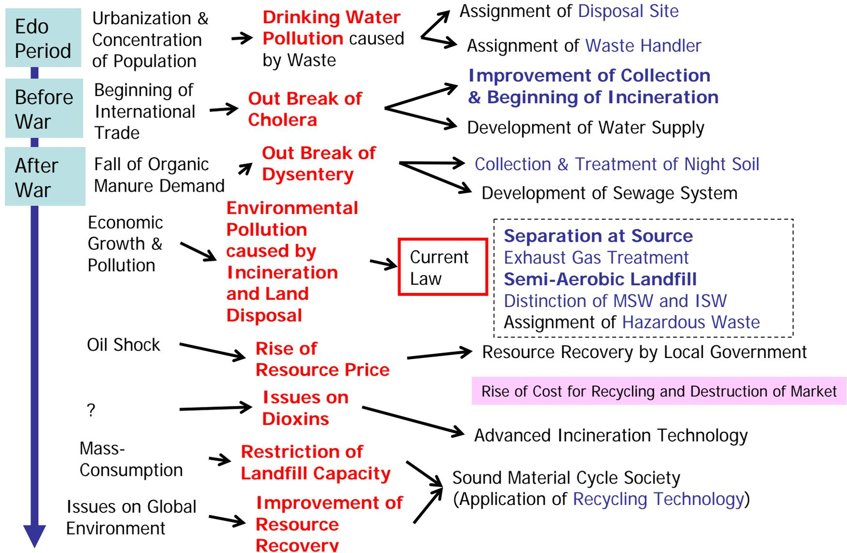
GHG emission from landfill sites has been **drastically reduced** by “Separation at Source”, “Intermediate Treatment (Incineration)” and “Semi-Aerobic Landfill”, which were originally introduced for improvement of public health and environment.
