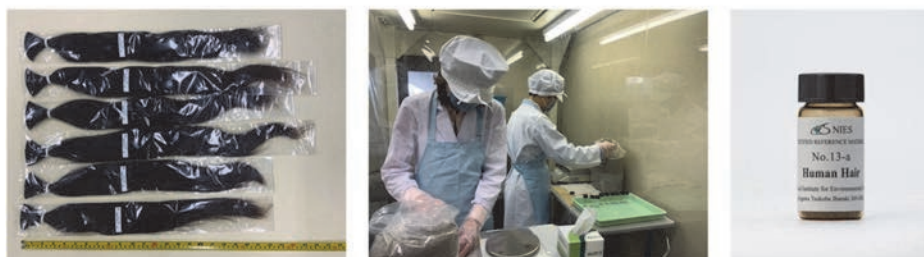
Fig. 3 Pictures of raw material, scalp hair (left), the bottling operation (middle), and the developed CRM (right).
