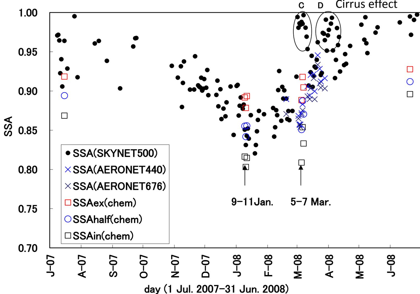
**SSAo by skyradiometer and SSAC by surface chemical compositions, assuming external (ex), half internal (half), and internal mixture (in). SSAC is only calculated for several cases, because the size distribution of atmospheric aerosols are used at Amami, not Phimai.**
