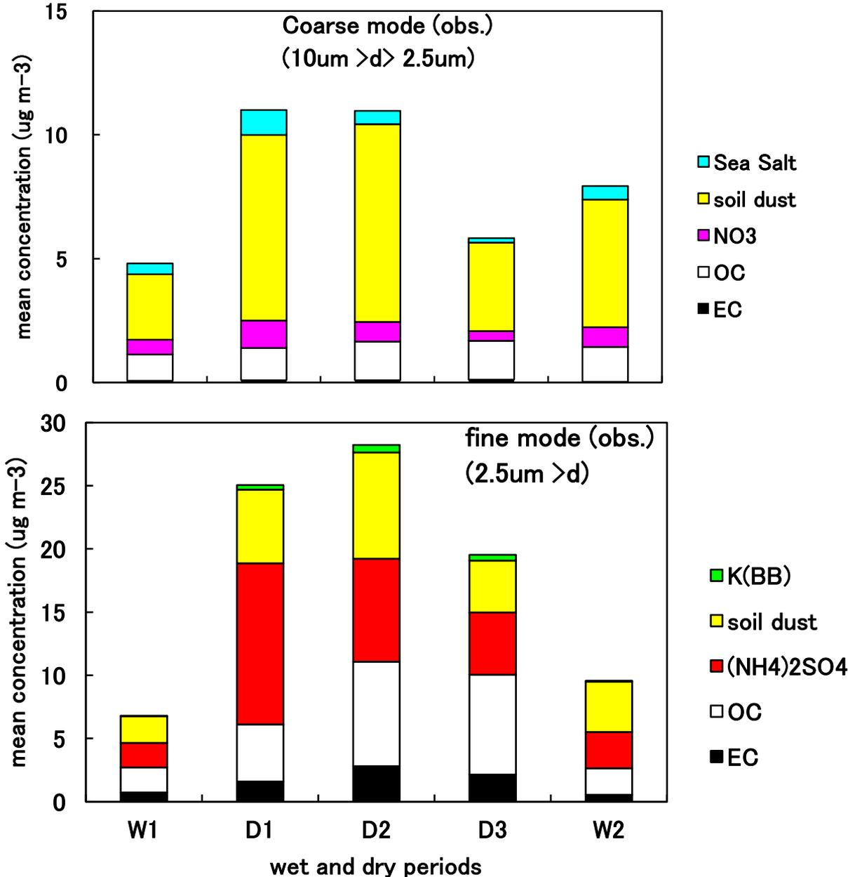
**Mean chemical composition for fine and coarse particles
