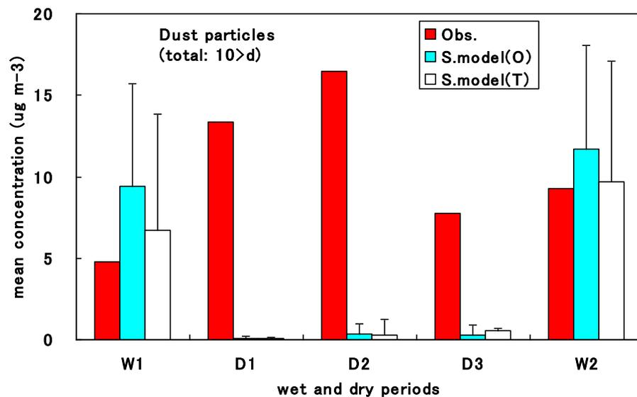
**4. Dusts: Large difference between the measurement and the model in the dry periods (SPRINTARS  $\ll$  Measurements)**
