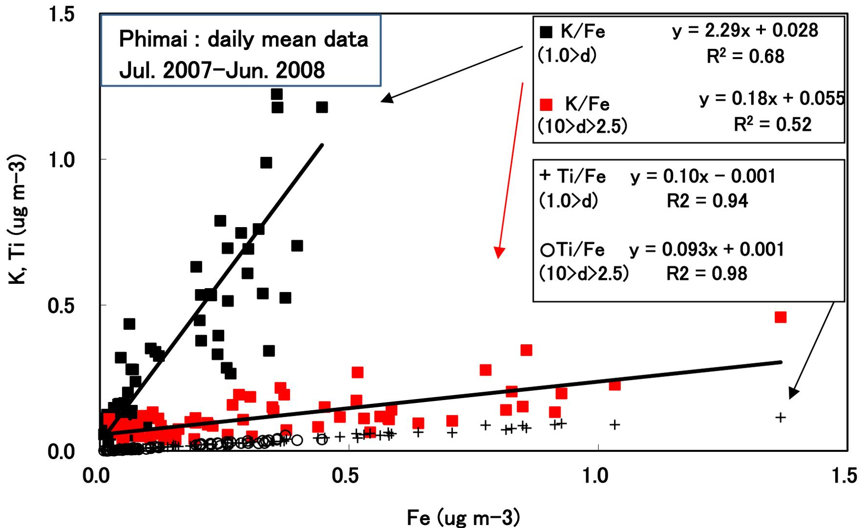
**Relationship for K/Fe and Ti/Fe in coarse particles and PM<sub>2.5</sub>
