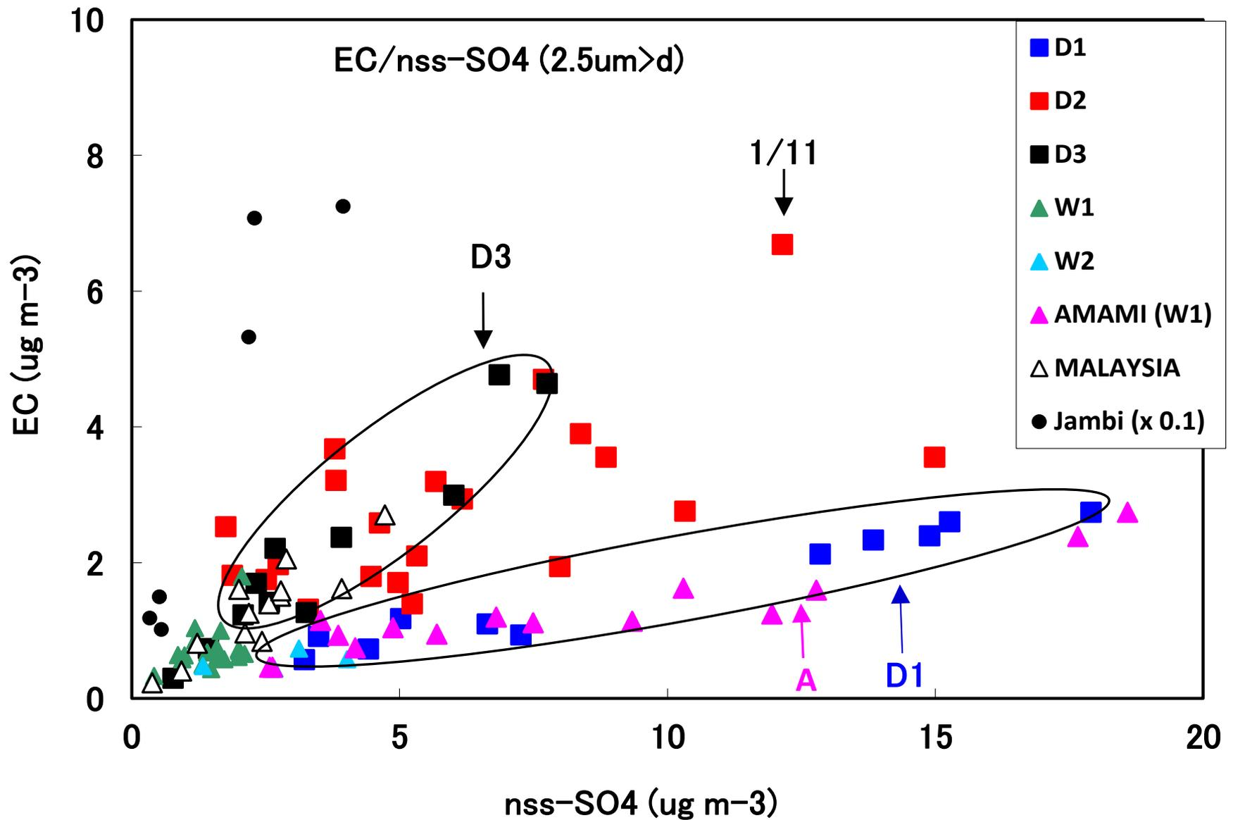
Scatter diagram between nss-SO4 and BC in PM2.5 from surface measurements (Phimai, Amami, Malaysia, Indonesia (Jambi))
