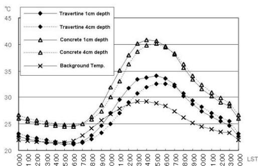
Fig. 6 Comparison of temperatures inside specimens in fine days (left)
