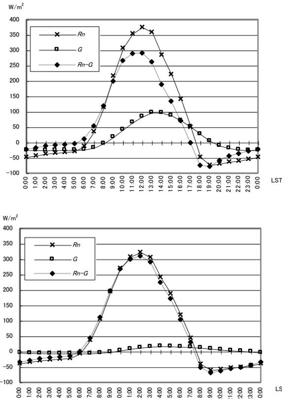
Fig. 9 Comparison of net radiation balance ( $R_n$ ), conductive heat flux at the bottom of specimens ( $G$ ) in fine days,  $R_n - G$
