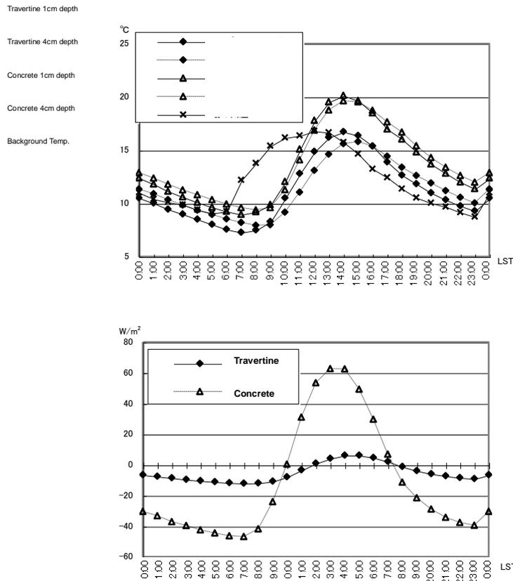
Fig. 10 Comparison of temperatures inside specimens in fine days (upper)
