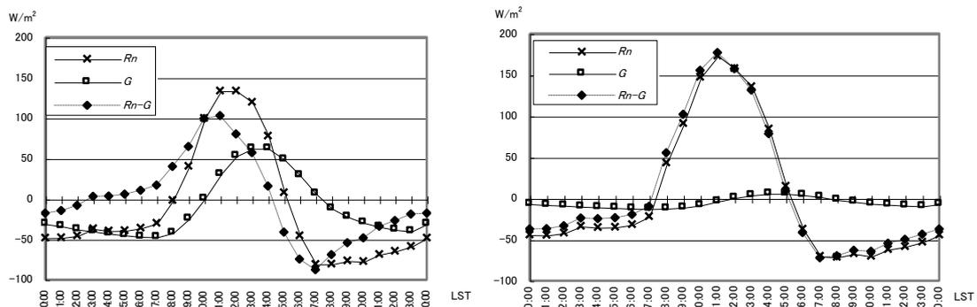
Fig. 13 Comparison of net radiation balance ( $R_n$ ), conductive heat flux at the bottom of specimens
