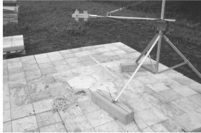
Fig. 4 Measurement of radiation balance above the specimens (left)
