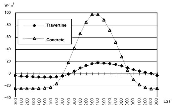
Fig. 7 Comparison of conductive heat flux at the bottom of specimens in fine days (right)
