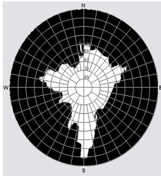
Fig. 5 Example of sky view photograph by fish-eye lens to generate data on buildings to be input to RayMan Model: Overlaid on Wulff-net to calculate SVF
