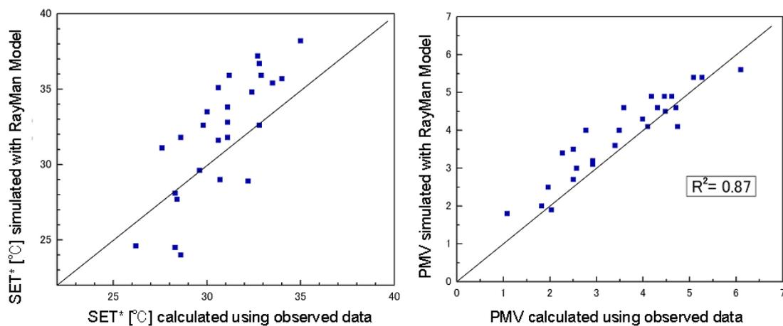
Fig. 6 Comparison between thermal comfort indices: calculated using observed data (x-axis) and simulated with RayMan Model (y-axis)
