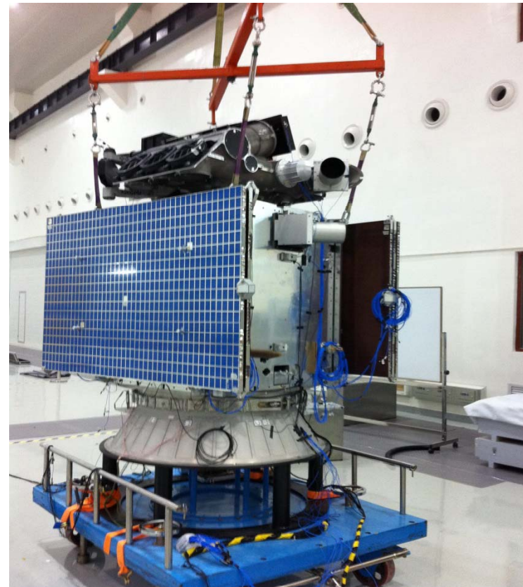
TanSat in the vibration and mechanical experiment
