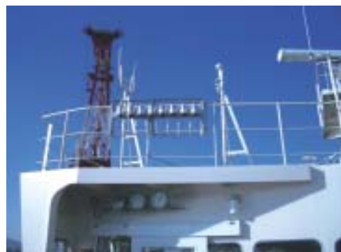
Atmospheric sample inlets for greenhouse gas measurement, installed above the wheelhouse of MS Trans Future 5
