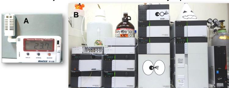
**Fig 3. (A) Data logger for temperature and relative humidity (B) High-performance liquid chromatography**
