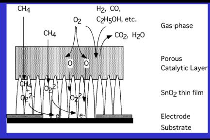
Conductiv R+O<sub>2</sub><sup>2</sup> → RO+2e ons are released; proportional to the amount of reduced gas
